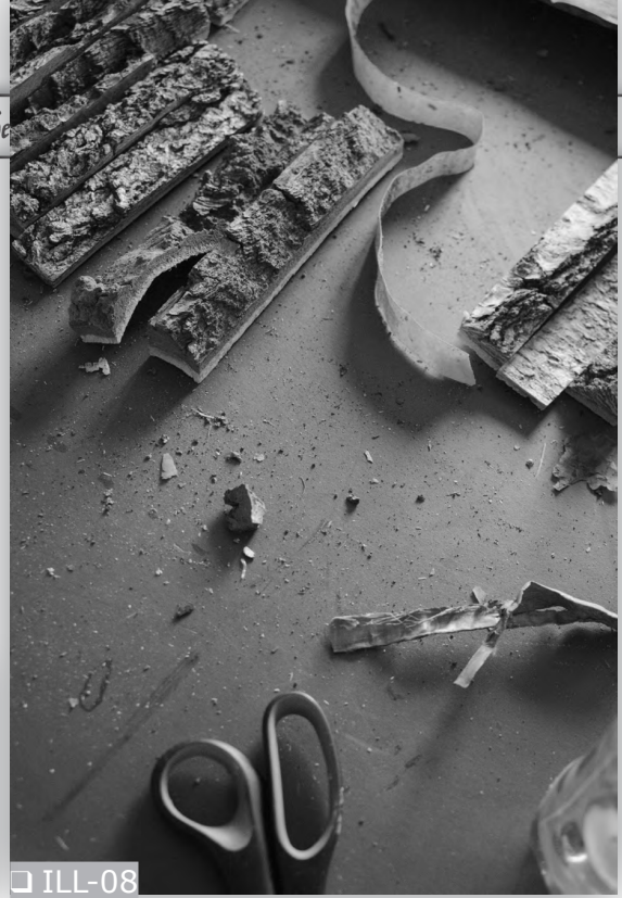
Oak bark and birch bark were cut into narrow strips against and along the fiber direction.
